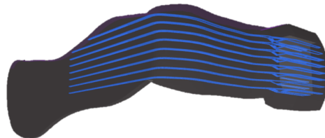
Figure 5: CAD model of the interior of the printed AFO displaying the layers of the carbon fiber
