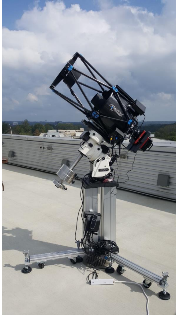
Figure 1: 14" PlaneWave telescope, AstroPhysics 1100GTO equatorial mount, and SBIG STXL-6303E camera [4]
